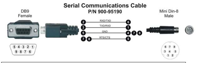
Note: To ensure proper operation, connect only properly wired RS-232 serial communications cables to the projector's control port.
